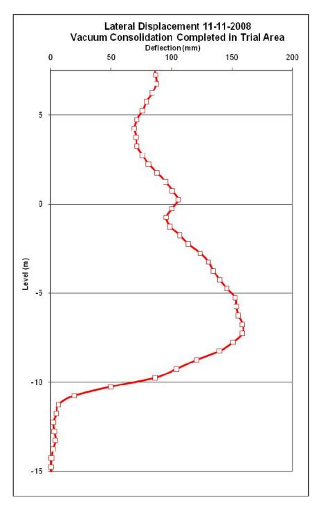
**Figure 9. Typical Inclinometer Readings**
