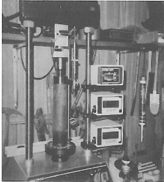
Figure 6. Core of Soilcrete Column
