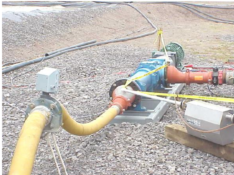
Figures 6. Pumping unit with density meter to the right and flow meter to the left.
