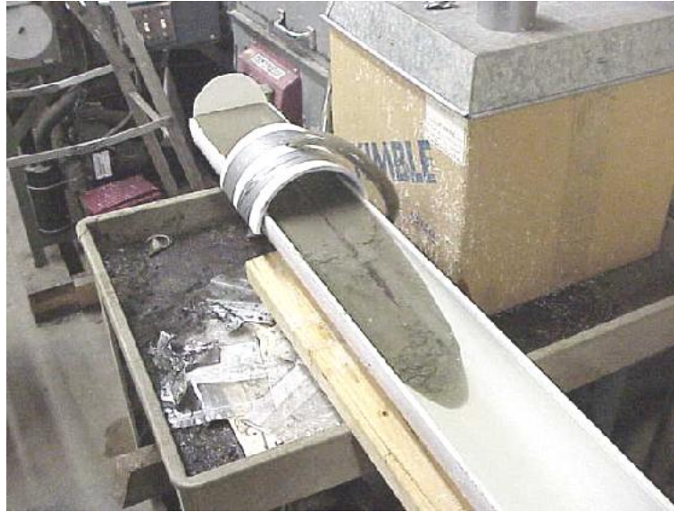
Figure 2. Model test of grout placement in a tunnel full of water
