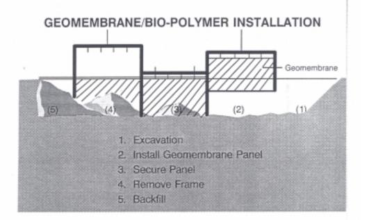
Figure 2. Sequence for Installation of Geomembrane in Bio-Polymer Trench
