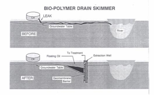
Figure 1. Schematic of Oil Skimmer Interceptor Trench
