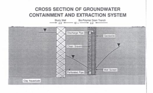
Figure 4. Cross Section of Groundwater Containment System
